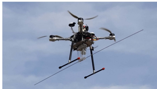
Fig. 3. UAV-mounted dipole hovering during the measurement.
