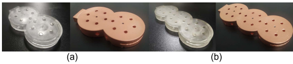
Fig. 12. Manufactured prototypes of the side-slot coaxial-resonator-based filtenna before and after Cu-plating. (a) Second order. (b) Third order.
