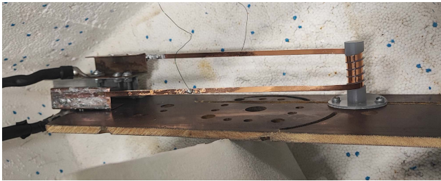
Fig. 4. F_5^5 former and sample holder in the cooling box during the short circuit test.
