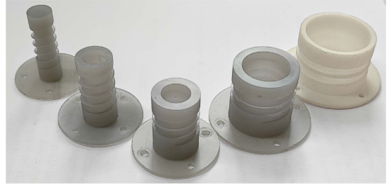
Fig. 2. 3D printed formers for I_c testing.
