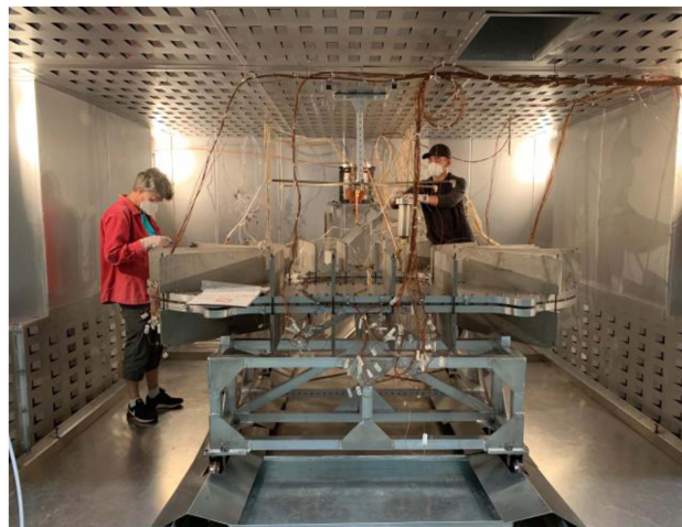
Fig. 14. TFMCO solder station at MIT showing a pancake VPI solder assembly inside a large convection oven.
