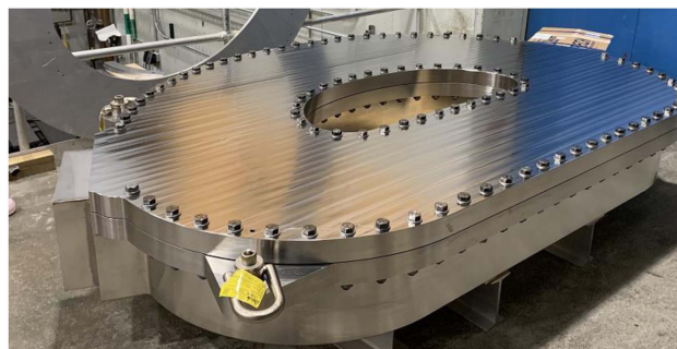
Fig. 18. Following installation of the WP, the structural case cover is bolted to the trough.
