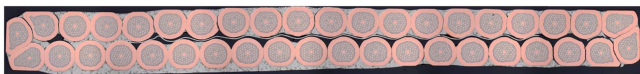
Fig. 3. Example cross-section (optical micrograph) of a Rutherford cable produced with the FalconD design using KAT DT wire before heat treatment.
