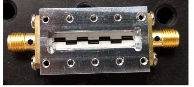
Fig. 6. Packaged notch filter with lid removed.
