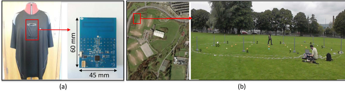
Fig. 1. (a) Purposely developed garment with mounting pocket at front central chest and the bodyworn wireless node used in the measurements; (b) satellite view and side view of the measurement environment showing the positions of base stations.
