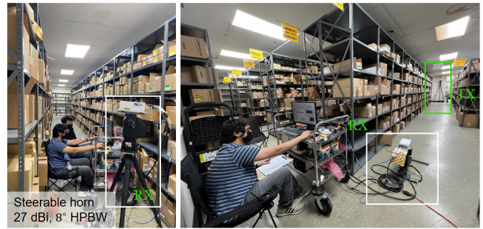
Fig. 5: Measurements in factory C. The TX was set at 2.5 m, and the RX was set at 1.5 m and 0.5 m.
