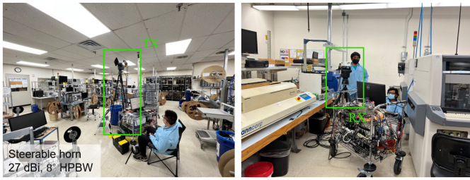
Fig. 3: Measurements in factory B. The TX was set at 2.5 m, and the RX was set at 1.5 m.
