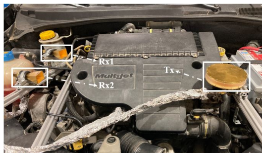
Fig. 2. Transmitter and receiver antennas in the engine compartment.
