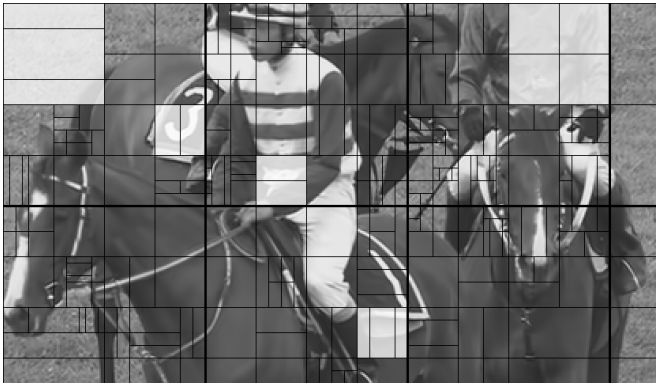
Fig. 1. Example of a picture partitioned into CUs, where VVC's five split patterns are highlighted (quaternary, horizontal binary, vertical binary, horizontal ternary, and vertical ternary). Thick lines represent CTU boundaries.
