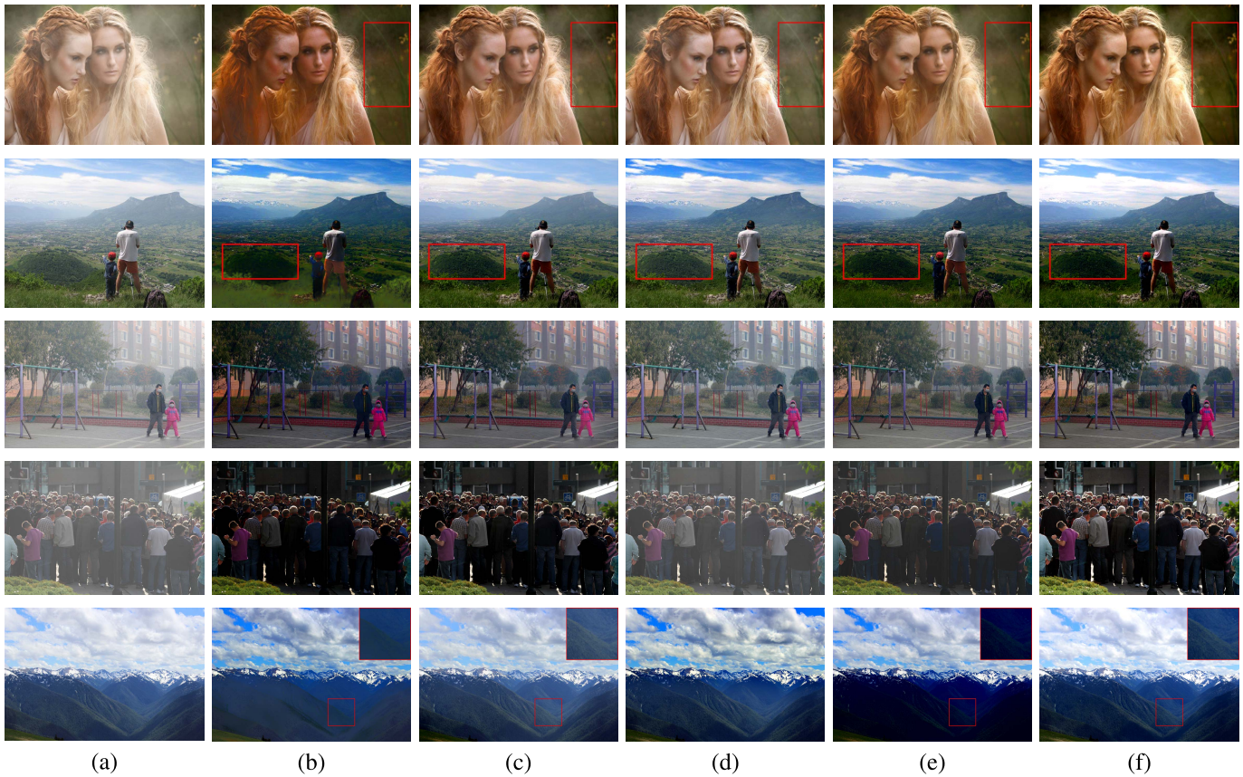
Fig. 11. Comparison of different methods on real-world images. (a) The hazy images. (b) CAP [30]. (c) DehazeNet [15]. (d) MSCNN [16]. (e) AOD-Net [20]. (f) HRGAN. (Red rectangles are used to highlight the improvements obtained by HRGAN. Red rectangles in the top-right corner is the zoom-in views).
