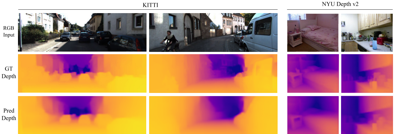
Fig. 1. METER depth map predictions (third-row) over the KITTI and NYU Depth v2 datasets. GT depth maps are resized to match METER output resolution. The depth maps are converted in RGB format with a perceptually uniform colormap (Plasma-reversed) extracted from the ground truth (second-row), for a better view.
