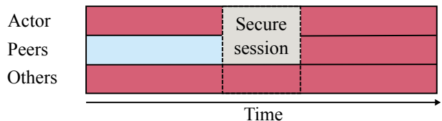
(c) Adversary model with KCI/AKC. Later works also consider adversaries that can compromise the actor’s long-term private key at any time, and showed that a secure session can still be achieved. In AKE literature, such protocols are said to offer resilience against Key Compromise Impersonation (KCI).
