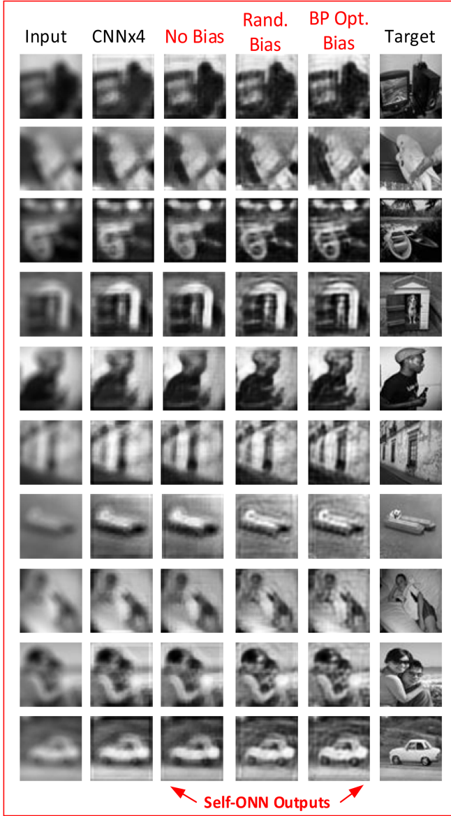
Fig. 6. Some typical original (target) and Disc-5 blurred (input) images and the corresponding outputs of the CNN \times 4 and the three Self-ONNs (with no, random and BP-optimized spatial bias) from the test partition.
