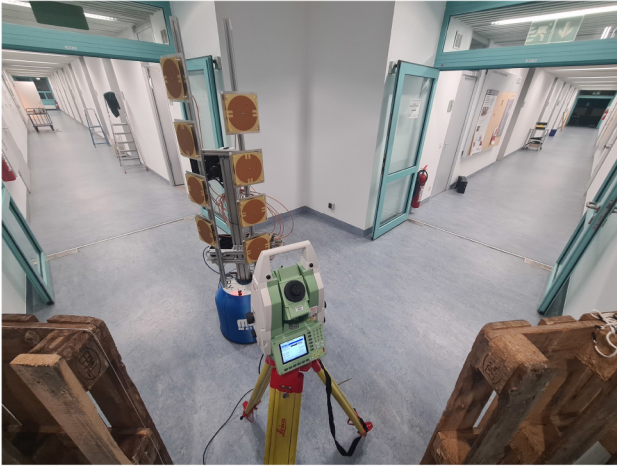
Fig. 2. Mobile robot platform with 4 \times 2 antenna array that drives in the corridor and is tracked by a Leica TS30 tachymeter.
