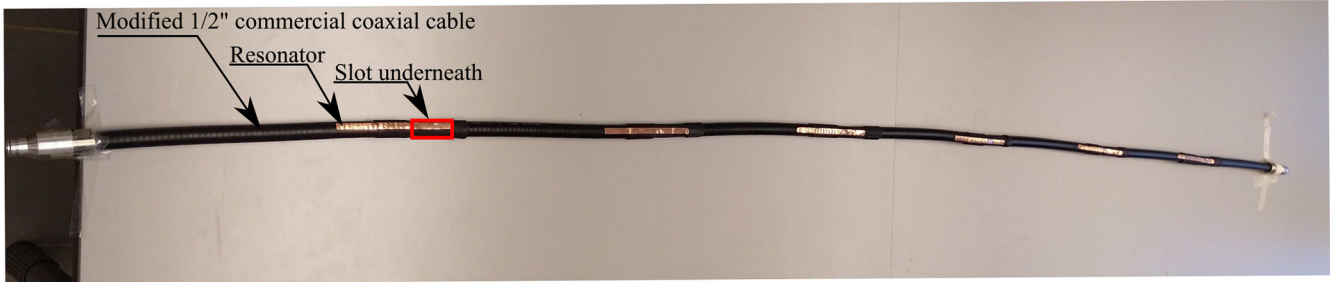
Fig. 4. Photograph of 2.1 m RCX with six slot-resonator pairs. Cable schematic can be found in Fig. 2 (Case 3), slot, and resonators dimensions in Table I.
