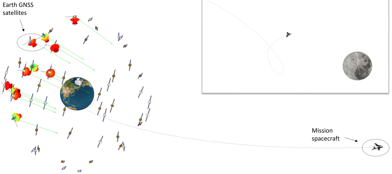
Fig. 2. Snapshot of the mission-case scenario as reproduced by the custom MATLAB ® -based mission planner and GNSS constellation simulator. Transmit-antenna radiation patterns are shown for satellites in radiometric visibility from the spacecraft. Vectors pointing towards the spacecraft are shown as well.
