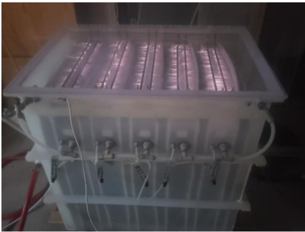
Fig. 5. Commercial 10-gpm water treatment system based on electrical discharge plasma (courtesy of Plasma Research Laboratory, Clarkson University).
