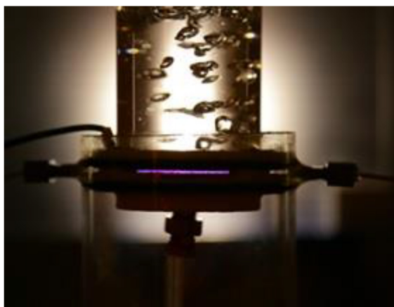
Fig. 4. DBD for nitrogen fixation in water. The plasma is in direct contact with the water surface. To increase the residence time and the surface area to volume ratio, air is flown through the plasma and bubbled into a 500-ml water column (courtesy of Plasma for Life Sciences Laboratory, North Carolina State University).
