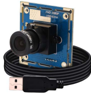
Fig. 3. Camera with the CMOS OV2710 image sensor installed in the vision-based unmanned kiosk.
