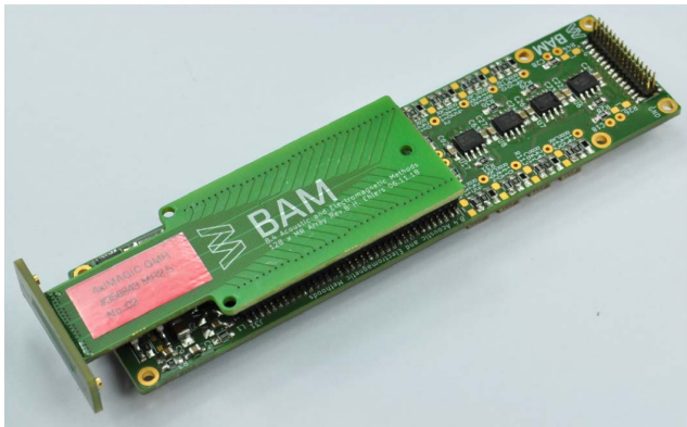
Fig. 5. MR probe with 128 MR elements mounted onto the multiplexer and amplifier PCB.
