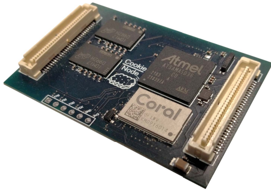
Fig. 2. Cookie IoT node with an EdgeTPU accelerator chip integrated.
