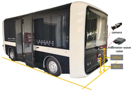
Fig. 7. Millimeter-wave radar and camera installation position diagram.
