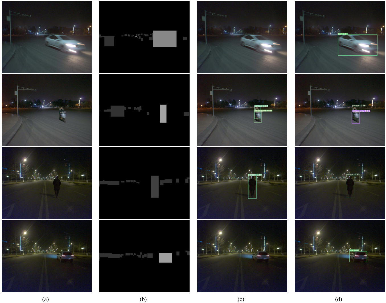
Fig. 12. Night scene detection effect. (a) Original camera image. (b) Radar mask map. (c) YOLOv5s test results. (d) MS-YOLOs test results.
