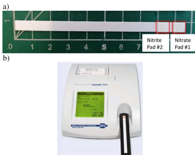
Fig. 1. a) Quantofix Nitrate 100 test strip with two test pads. b) Quantofix Relax test strip measuring device.
