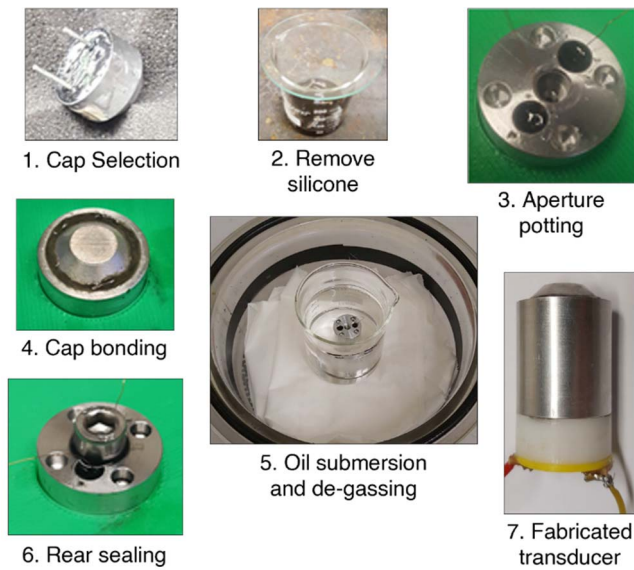
Fig. 3. A simplified fabrication process for an OFFUT. Note that Step 5 shows the vacuum chamber with the sealing lid removed for clarity. The fabricated transducer shown in Step 7 is complete with acrylonitrile butadiene styrene (ABS) plastic strain relief.
