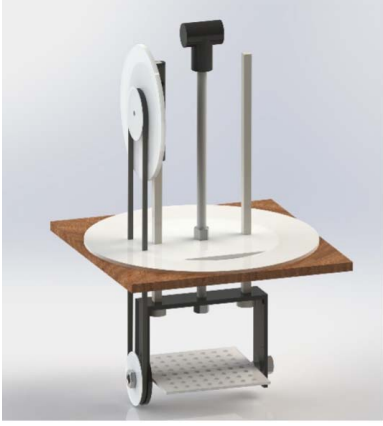
Fig. 3. Target orientation manipulator capable of rotating objects around one axis.
