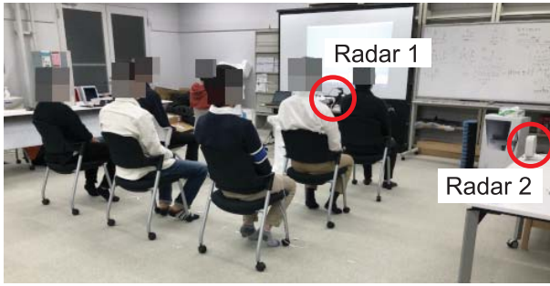
Fig. 3. Measurement setup with the seven seated participants shown with belt-type respirometer devices on their upper torsos in scenario 1.
