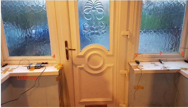
Fig. 6. The receiving nodes are located from both sides of the doorway and connected via USB hub to a laptop. The transmitting node is located indoor at the same height approximately 2 meters from the door.
