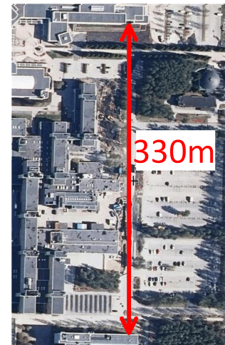
Fig. 22. Measured signal strength from the wall of a building at a distance of \sim 330\text{m} . A 1550nm laser pulse with a width of 20ns and peak power of \sim 4\text{W} and a receiver aperture of 20mm were used in the measurements.
