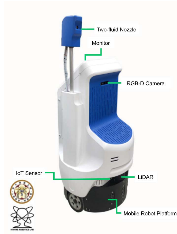
Fig. 2. The hardware for the smart sterilization robot system.
