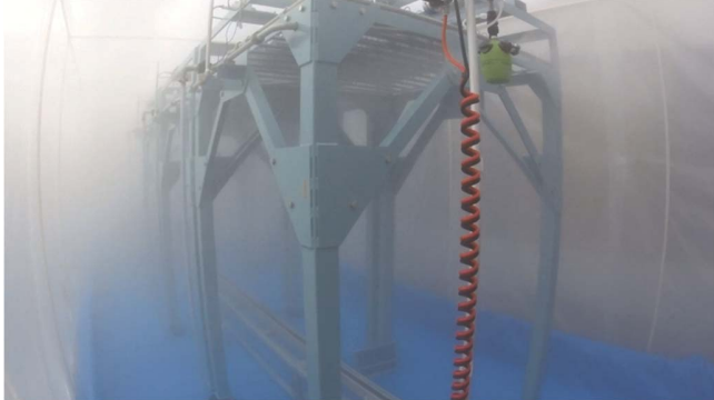
Fig. 4. The thickest fog environment reproducible with the simulator. The transmittance at 5 m distance is less than 2%, T_5 \leq 0.02 . The yellow-green spindle in the front top of the image is one of the fog generators. The large pale-green steel frames are parts of a rainfall apparatus, not related to this experiment.
