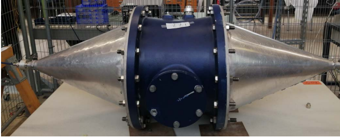
Fig. 1. Picture of the Testbench used to characterize PD antennas in GIS.
