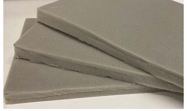
Fig. 4. Polymer foam samples with the thickness of 30 mm.
