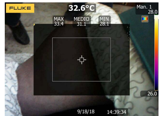
Fig. 9. Leg captured by the infrared sensor during verticalization (standing up) position while reaching the 45° angular position. Temperatures are reported in the pictures.
