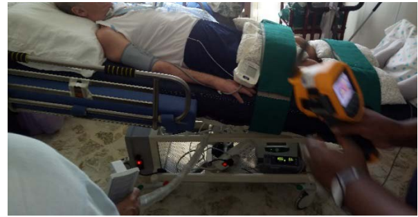
Fig. 4. Instrumentation and sensing systems beneath the patient bed, and infrared camera.
