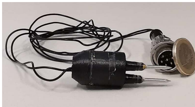
Fig. 2. The stainless-steel double-needle sensor.
