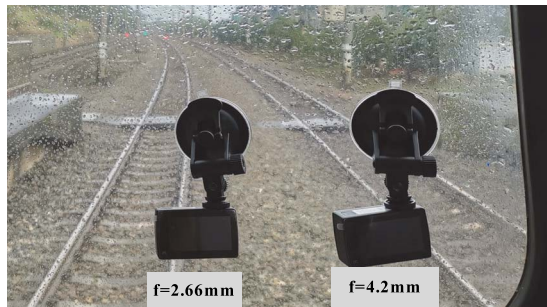
Fig. 14. Two cameras with different focal lengths installed on a train.
