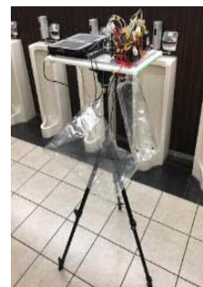
Fig. 11. Field test in a restroom. The sensor materials used were made from mixture of CB and GC materials (without the hydrophobic polymer). The materials were annealed.
