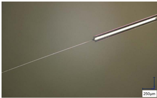
Fig. 5. The cantilevered fiber obtained via etching process (scale bar = 250 μm).
