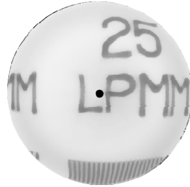
Fig. 17. Reconstructed image of the resolution target corresponding to 25lp/mm.
