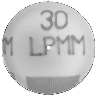
Fig. 18. Acquired image of the resolution target at 30lp/mm.
