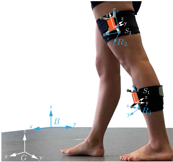
Fig. 1. Experimental setup: Two inertial sensors are attached to thigh and shank body segments. Reference coordinate frames (blue) R_1 and R_2 are formed by clusters of optical markers that follow the movements of inertial sensor coordinate frames (white) S_1 and S_2 . Sensor orientations are estimated with respect to a global coordinate reference frame G and reference orientations are obtained with respect to a Vicon base coordinate frame B .
