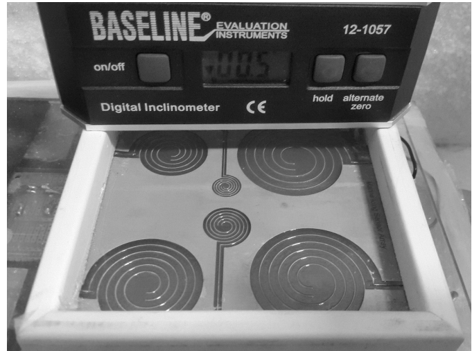
Fig. 7. Sensor Leveling prior to the Experiment.
