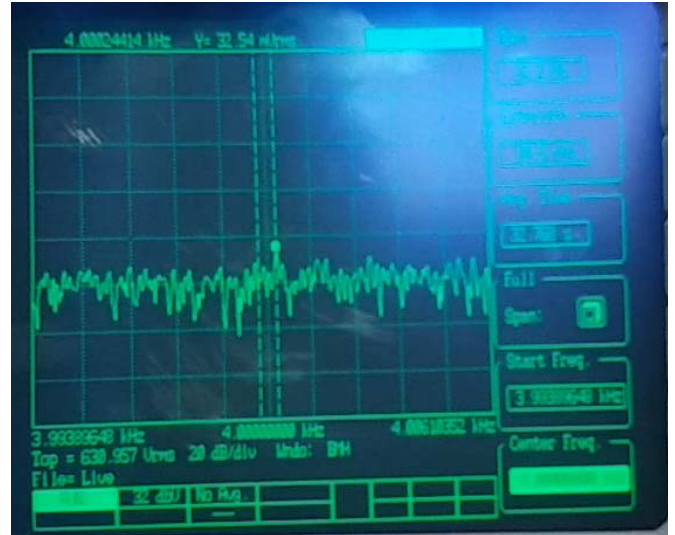
Fig. 18. The noise floor of the system.
