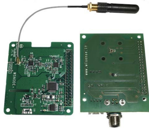
Fig. 10. Photo of the hardware components of the developed Sensor Node: Core Unit (left) and Sensing Unit (right).
