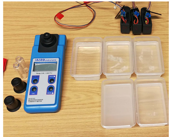
Fig. 3. Prepared solution as water samples, the concentration of fat particulates within each sample was changed by mixing the particles with distilled water. HI 93703, as a reference meter, was used to determine the turbidity of each sample.
