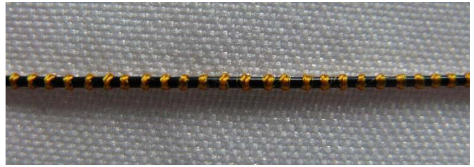
Fig. 1. Sewn on insulated conductor (conductor diameter 0.52 mm, stitch pitch of 1 mm).
