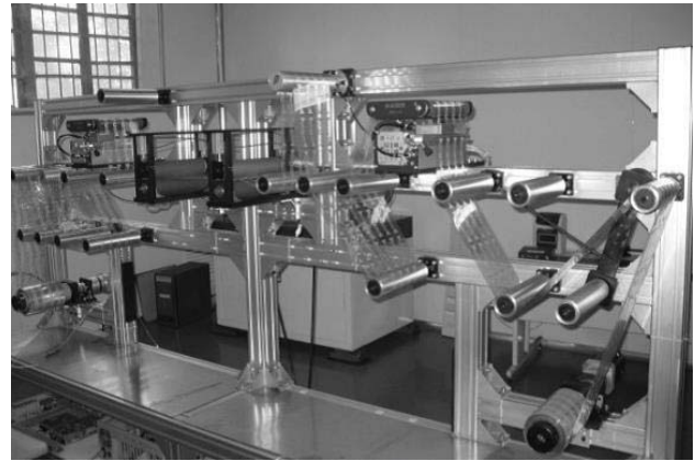
Fig. 20. Image of a Roll-to-Roll (R2R) setup in a clean room environment with different printing process units installed in the production line [3].
