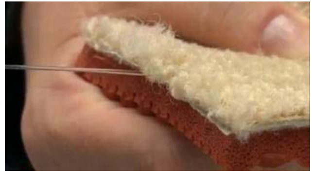
Fig. 5. A cut-out of the sensor head showing the cross section with the top pile carpet, the position of the POF layer and the underlay.
