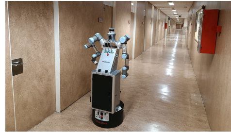
Fig. 5. Example scenario in which ADAM was teleoperated to capture data. The 3-D sensor is located in its uppermost part.
