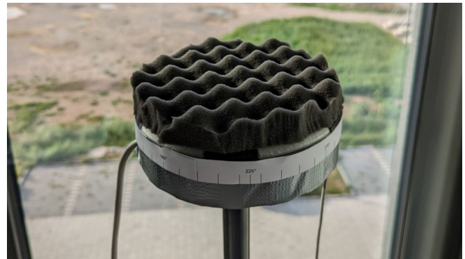
Fig. 4. UCA microphone array with a windscreen for outdoor usage. Details of the employed algorithms can be found in [45].
