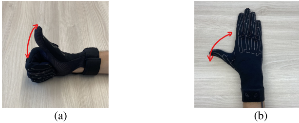
Fig. 6. Vertical thumb movement [11] and newly proposed alternative for the thumb CMC flexion. (a) Vertical thumb motion. (b) New thumb flexion.
