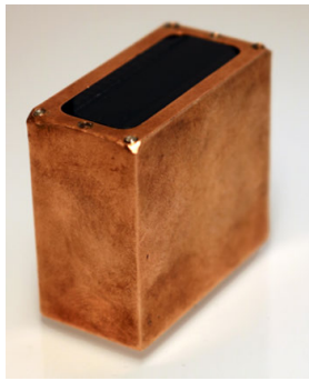
Fig. 12. PET block placed in the enclosure of medium-sized sensor made of copper.
