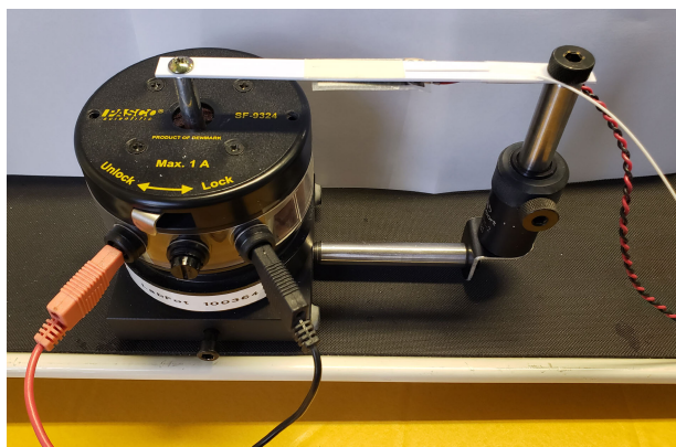
Fig. 6. Experimental setup of the sensor to apply the vibration frequency.
